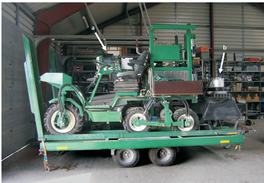
Phot. 3. A computer-driven tractor for fungicide treatment of small plots: a – computer, b – six containers for pesticides (photo by M. Maňka)
